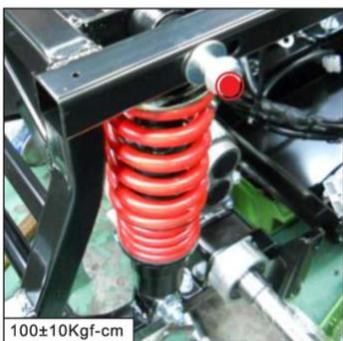
3. Remove the rear shock absorber lower fixing screw set (M10 x 45L x 1pcs).
