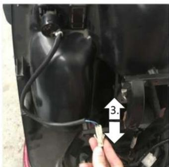
4. Remove the main power switch set from the slot.
