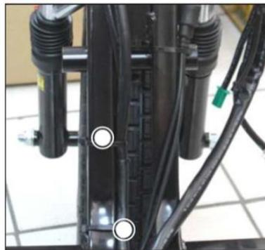
7. The main line passes through the groove at the bottom of the frame. Please directly pull it away from the groove.
