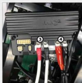
After reassembling or replacing the controller, please confirm to connect the connector and the connector screw, so as to avoid falling off, causing the abnormality of the scooter.
