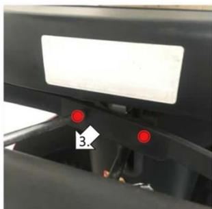
4. Remove the head steering lever back shroud clamping screws (M4 x12L x2pcs).
