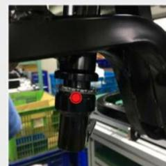
If the steel bead set needs to be reassembled or replaced, it is recommended to apply a small amount of grease to the upper and lower steel bead sets for lubrication.
