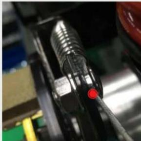
The other end of the brake cable will be connected to the head brake handle. If the end wiring is in normal condition, it may be that the head brake handle is abnormally connected.
