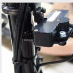
Step 6. For the two fixing straps, one for fixing the brake cable and the speedometer wiring (loosen and fix), and the other for fixing the main line (loosen and fix).
