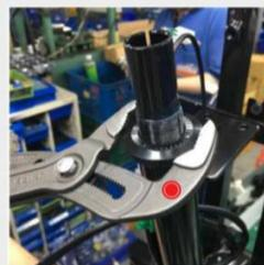
There is a set of steel beads at the bottom of the center bar. Please pay attention to avoid falling or missing when disassembling/reassembling. The beads should be placed at the direction of upwards.
