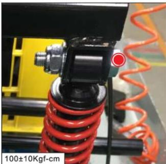
4. Remove the front shock absorber lower fixing screw set (M10 x 45L x 1pcs).
