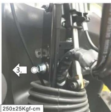
4. Remove the screw set (M6 x 30L x 1pcs) that connects the steering lever to the frame.
