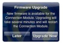
**DO NOT CYCLE THE POWER** during the upgrade process, even if the screen shows "unable to connect" and advises you to cycle the power. The connection will automatically resume after the upgrade process is complete.
