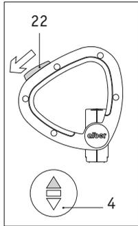
Pushing the direction of travel switch [22] forwards activates “Descending staircase”.
