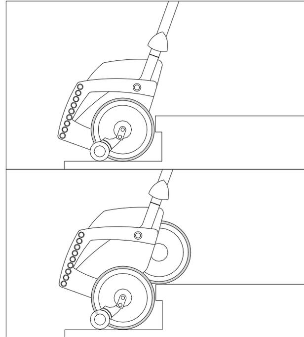
**!** During the climbing process always pull the scalamobil towards you. Also the scalamobil plus wheelchair needs to remain in the same tilted, balanced position all the time. Never release the grips of the scalamobil!
