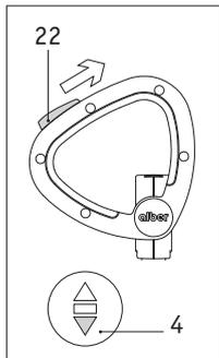
Pushing the direction of travel switch [22] backwards activates “Ascending staircase”.
