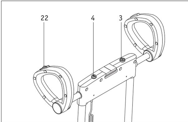
The scalamobil is switched on or off by pressing the On/Off button [3]. When switching on the display element [4] simultaneously shows the last direction of travel selected on the direction of travel switch [22] and the state of charge of the battery.
