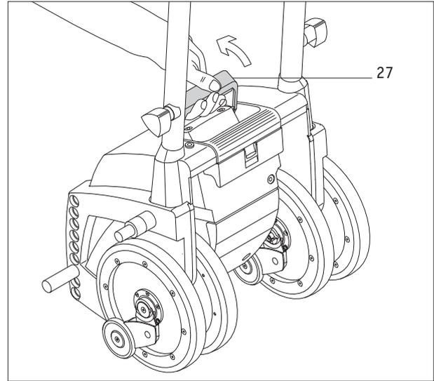
After you have removed the handle as described in the last chapter, you can fold out the carrying handle [27] that is integrated into the housing, in order to be able to transport the scalamobil.
