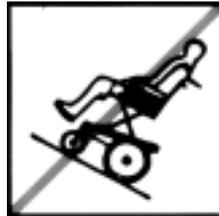
**Do not drive up or down slopes when the lifter is raised!**
