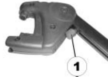
The rubber stop can be screwed in or out (A) or pushed up or down (B).
