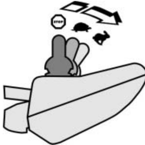
The further the joystick is moved in a particular direction, the more dynamically the wheelchair reacts.
