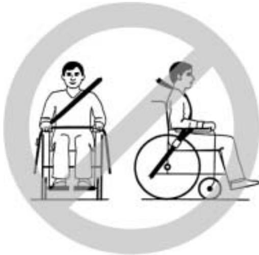
Seat belts may not be held at a distance from the user's body using parts of the wheelchair such as armrests or wheels.
