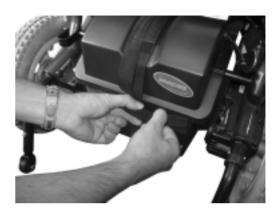
• Remove battery cable connecting plugs on both sides (the figure only shows the right-hand side).
