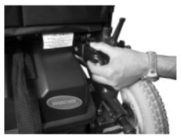
• Pull the rear battery box out towards the back.
