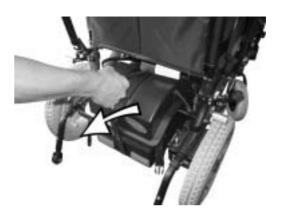
• Open the battery retaining strap velcro fastening.
