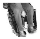
Unlock the legrest and swivel outward. The calf plate swivels backward on its own.
