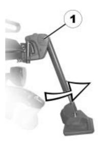
• Use the open-ended spanner to loosen the counternut (1).
