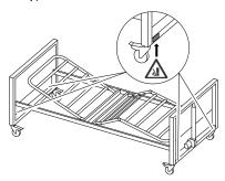
Place the four foot squeezing warning labels (delivered separately) on the lower sides of the bed ends near the castors.
