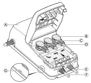
The control box (A) is provided with a label with symbols showing where to connect the motor plugs:
