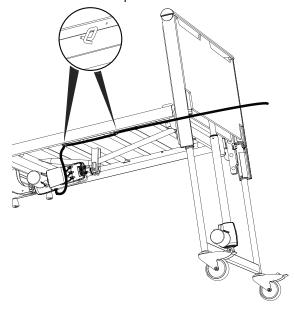
11. Before taking the bed into use, check that all parts run smoothly and that no motor cables are hanging on the floor or being squeezed while moving bed sections.
