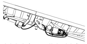
7. Guide the head Hi/Lo motor cable through the frame hooks on the side of the bed and the end of the coiled part on the bed end hook.
