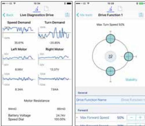
Professionals can now configure powerchairs quickly and intuitively to each individual thanks to the revolutionary programming interface built into **LINX**.
