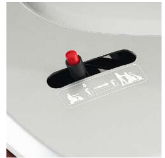
Two-step disengaging lever Prevents the scooter from accidentally free-wheeling.
