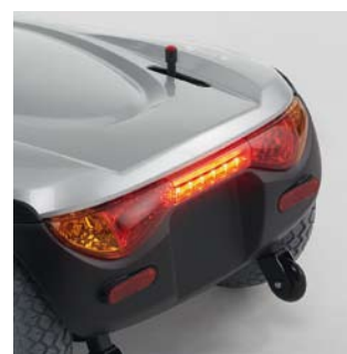
Brake light Heavy duty brake lighting warns people that the scooter is slowing down.
