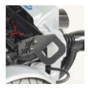
**Car Fixation** Four point tie-down points allow safe transportation in a car. \* Crash tested according to ISO 7176, part 19.
