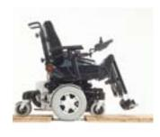
Increased traction The innovative Walking Beam enhances grip and provides better traction.
