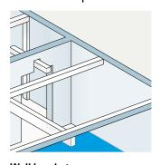
Wall bracket To install the track in a free span. The tracks are mounted at the ends.
